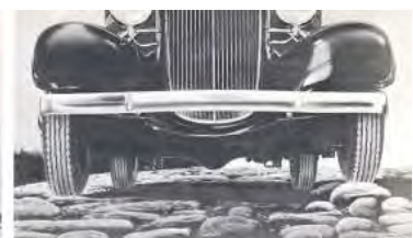
Knee-Action obsoletes solid front axle, 1934
